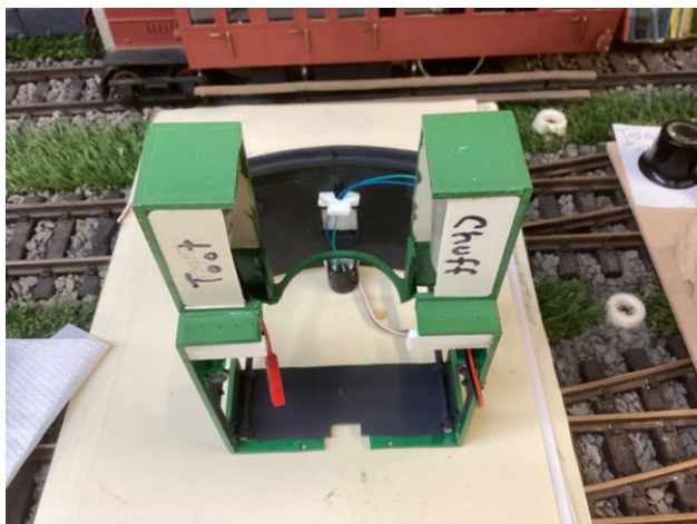
The Tail light wiring is in place ready to join to the motor feed wires.
