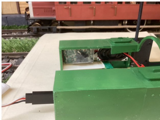
Sound cards, amplifiers and speakers subassembly units are attached with double sided sticky tape.
