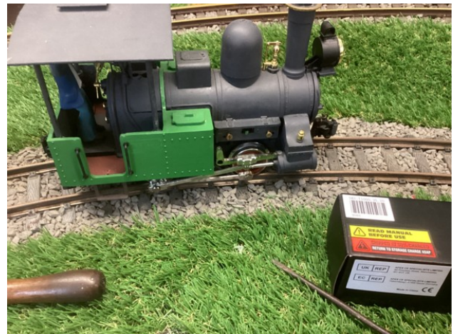
OTTO photo as initially modified with short side tanks, open cab, zero lights & trigger type Tx/Rx.
