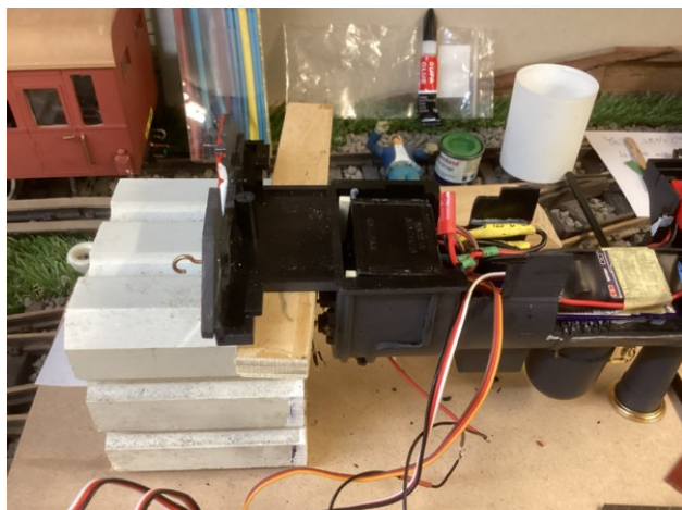
The standard servo, CAM and DPDT switch was fouling with wires in firebox so it was enclosed. This presented a new fouling location where the firebox straddled the brown plastic motor block. The enclosed direction servo unit was now somewhat bigger and needed to be flush with footplate, So, some material was cut away at the rear of gear/motor box.
