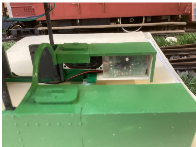
The Tail light wiring is in place ready to join to the motor feed wires.
